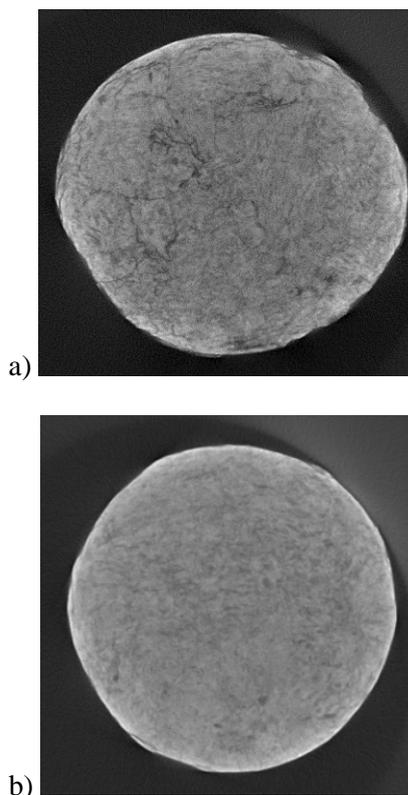
**Figure 6 – Cross-section of the sample for a) 1 stroke of the press, b) 8 strokes of the press**
