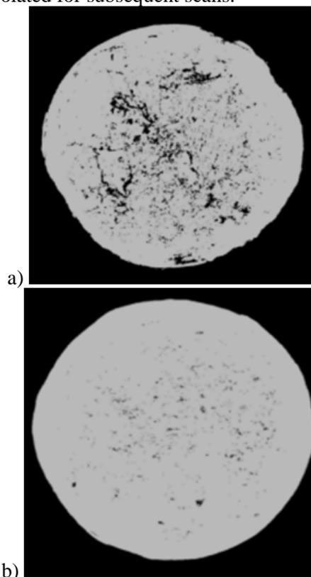
**Figure 7 – Cross-section of the sample after threshold for a) 1 stroke of the press, b) 8 strokes of the press**
