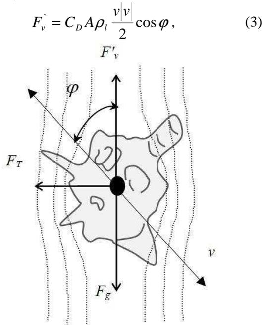
**Figure 4 – Forces acting on a star-shaped particle**
