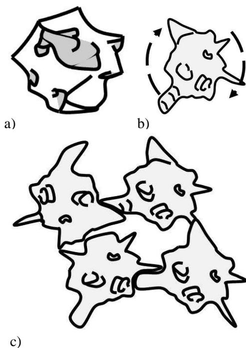
**Figure 2 – Types of floc structure a) complex flocs b) star-shaped c) agglomerates**
