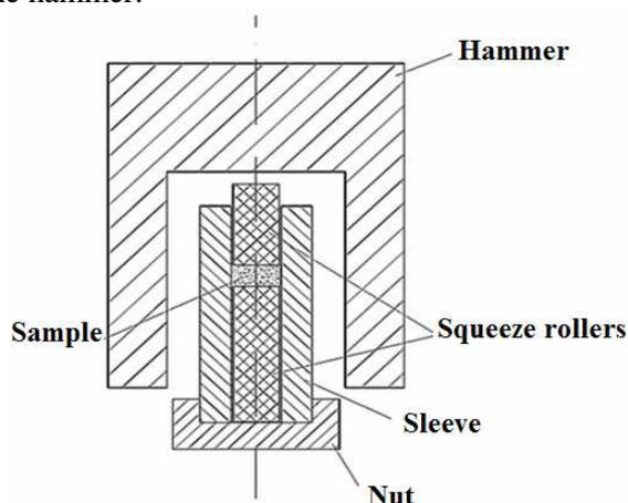
**Figure 5 – Scheme of the press impact**
