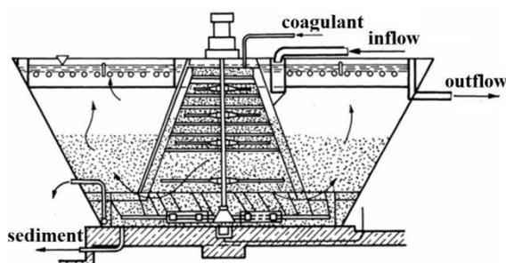
**Figure 1 – . Reactor clarifier "Precipitator"**
