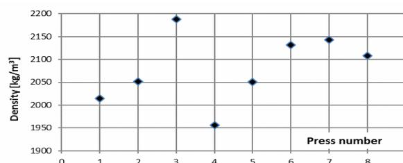
**Figure 9 – Relation between the sediment density and the number of strokes of the hammer**
